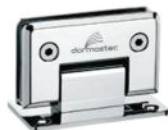
DSH-1 H/P Wall to Glass 90° Off Set Hinge Material : Forged Brass/SS 304/Zinc Door Thickness : 8mm - 12mm Finish : Matt & Chrome Plated
