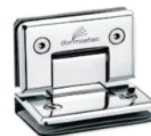
DSH-3 Glass to Glass 90° Off Set Hinge Material : Forged Brass/SS 304/Zinc Door Thickness : 8mm - 12mm Finish : Matt & Chrome Plated
