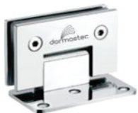
DSH-2A Wall to Glass 90° Off Set Hinge Material : Forged Brass/SS 304/Zinc Door Thickness : 8mm - 12mm Finish : Matt & Chrome Plated
