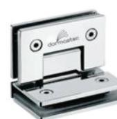
DSH-3A Glass to Glass 90° Off Set Hinge Material : Forged Brass/SS 304/Zinc Door Thickness : 8mm - 12mm Finish : Matt & Chrome Plated
